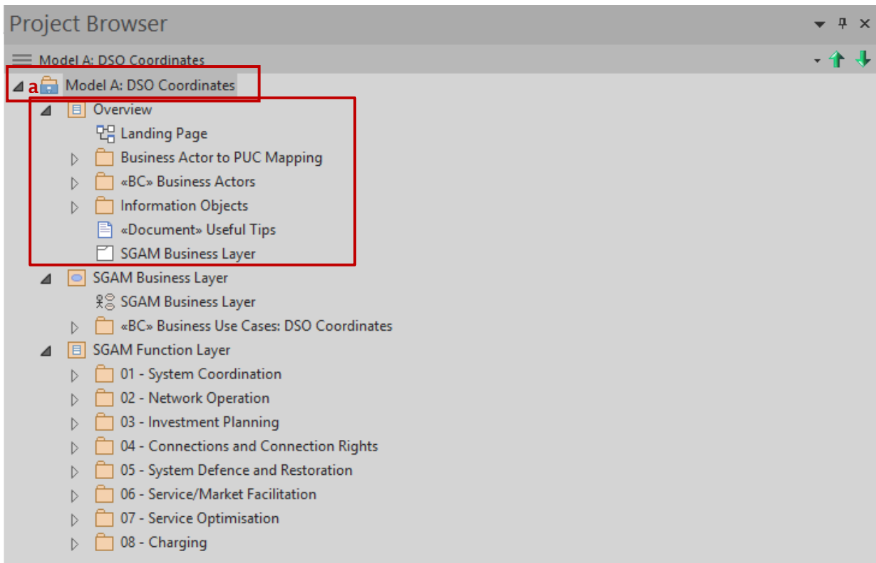
Figure 9: Project Browser showing the hierarchy of Packages beneath the model Root Node (a).
